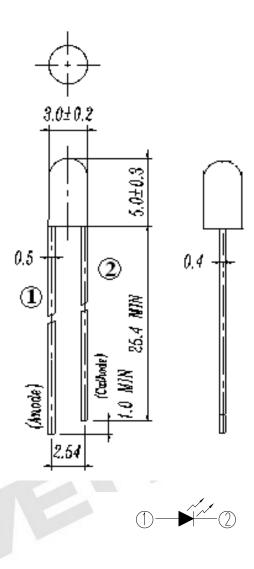
Note: Tolerances unless dimensions ±0.25mm
